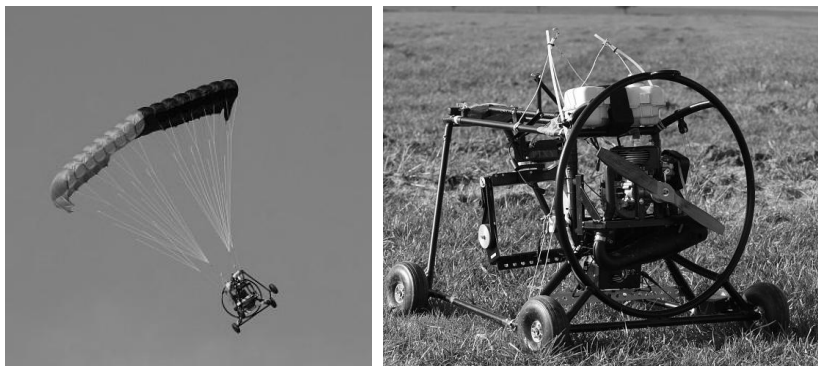
Fig. 2: Drone PIXY model. Left: the model during a flight. Right: detail of the engine part.
